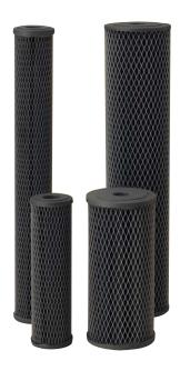
Pentair<sup>‡</sup> Pentek<sup>‡</sup> NCP Series Cartridges are constructed from a carbonimpregnated non-cellulose media. They offer sediment filtration, as well as taste, odor and chlorine taste & odor reduction in one cartridge. Unlike cellulose cartridges, NCP Series Cartridges can be used for municipal and non-chlorinated water applications.
